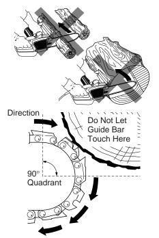
Figure 1 - Kickback Hazard Example: Do Not Let Nose of Guide Bar Touch Object While Chain is Moving
